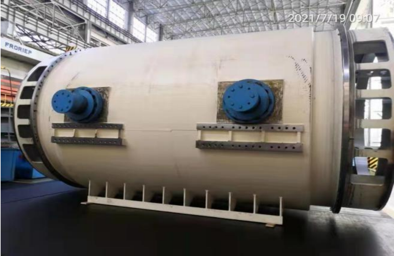
Paint Inspection of stator frame of #2 generator equipment
