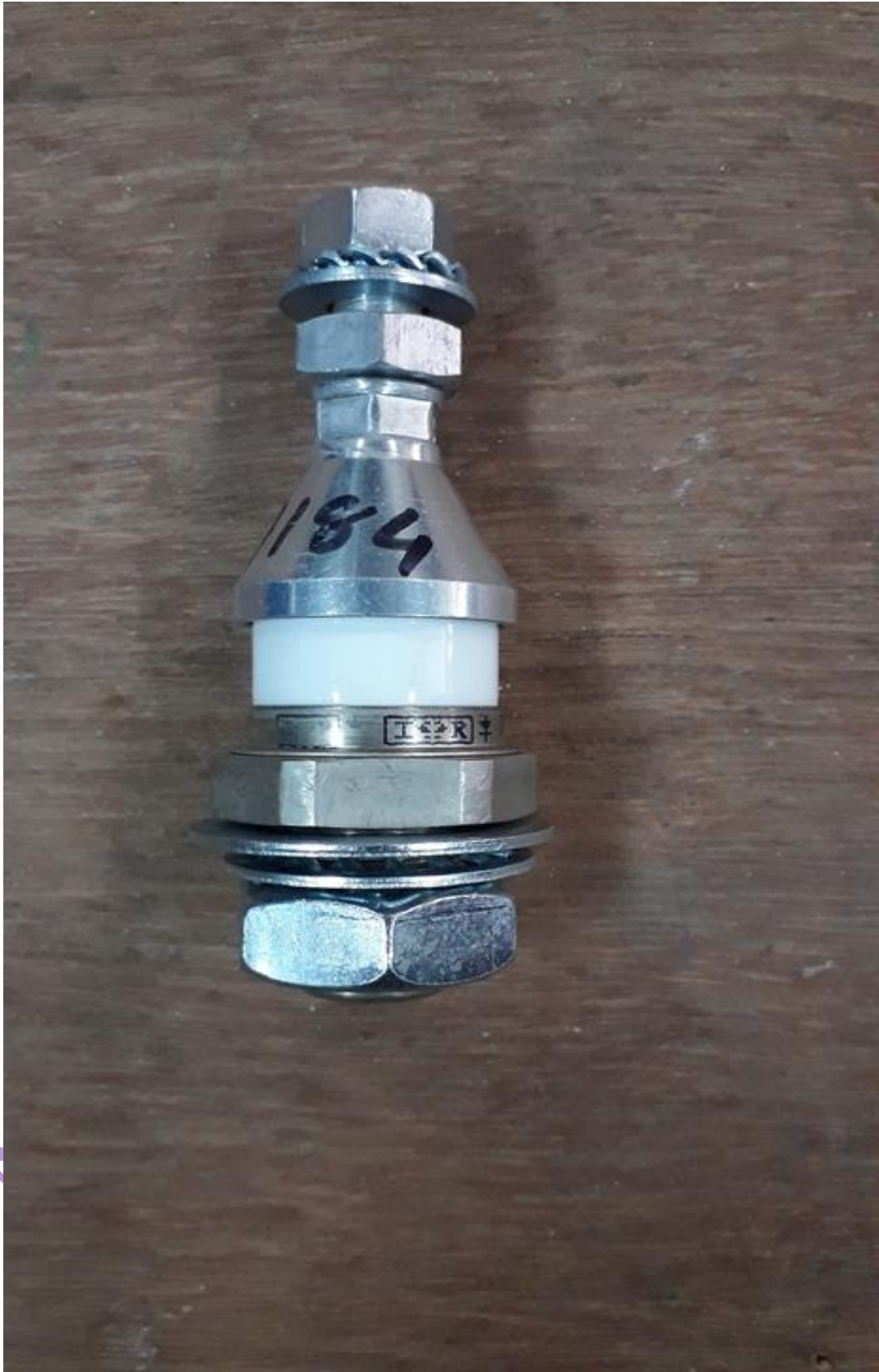
Fig: Existing Generator Diode Image.
